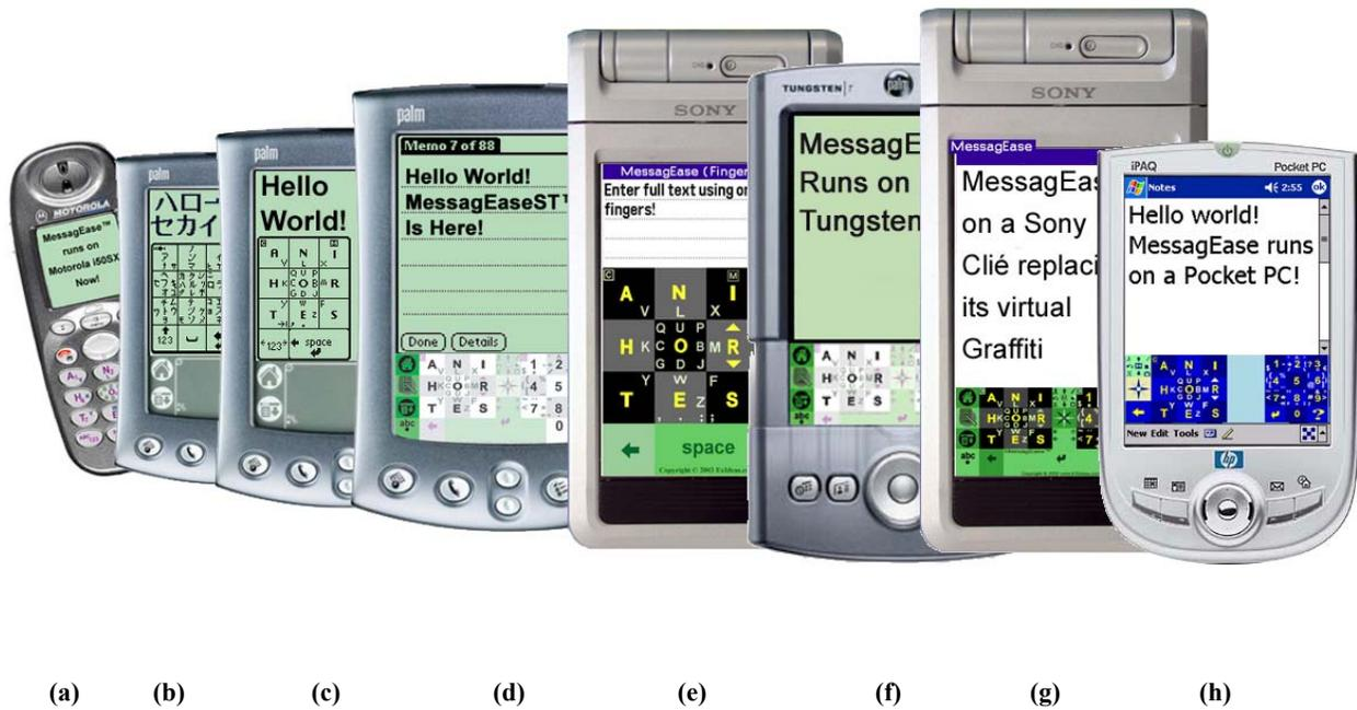
Figure 7. Current implementations of MessageEase: (a) Hard-key implementation for a cell phone, (b) Japanese (Katakana), (c) On-screen keyboard for Palm, (d) Graffiti replacement for Palm, (e) large keyboard operable with a single finger on a Sony Clié, (f) replacing the keyboard for Tungsten T, (g) with virtual Graffiti on a Sony Clié, and (h) MessageEase keyboard for Pocket PC.
